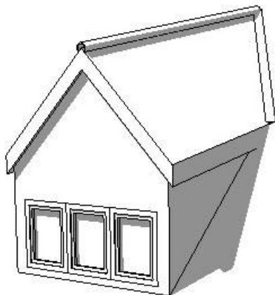
Dormer roof with side walls
