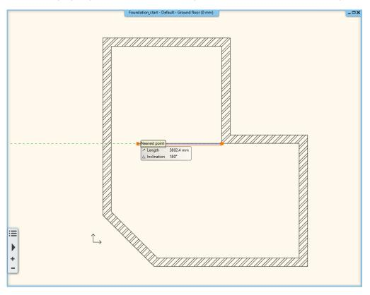
Move the mouse to the left horizontally. Now check the appearing virtual wall represented by an orange and blue line.
