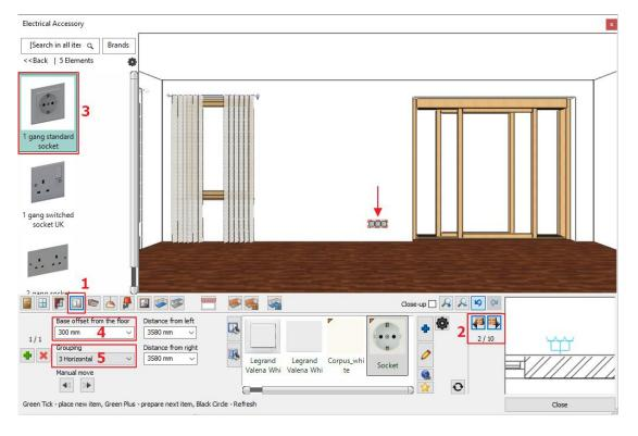
Place a single-gang socket on the wall with length 1900 mm next to the sliding door.
