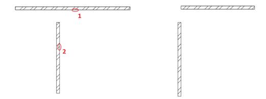
The wall segment which extends over the intersection will be modified.
