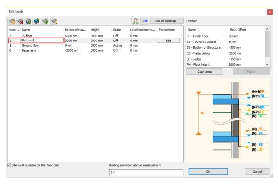
At the moment we can see the recently created ground floor level content such as walls, slab. This building has a flat roof, which can be drawn on other levels too. Right now it is hands-on tool the "copy other floor". To learn how to use it please do the followings:
