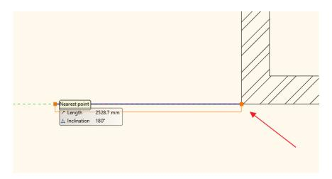
For now, we need the wall thickness to be above the blue reference line, so that the partition wall and the neighbouring main wall will share the same line. We have to switch the reference line. In the right top corner of the work area appears a floating menu with these commands you can execute the modification..
