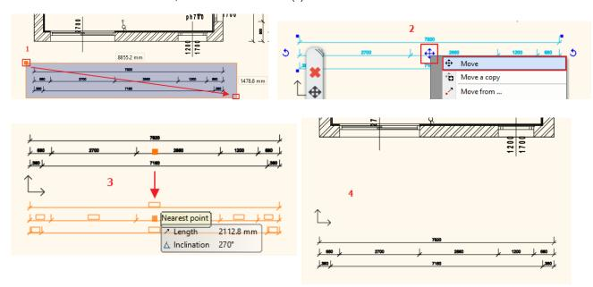
• Move the dimension lines to the desired position, ensuring that the values don't slip away from the dimensioned elements and then click on the ideal position (3).
