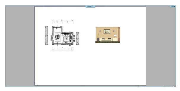
As described above, you can copy the dimensioned wall elevation view on the page by 1:50 scale factor. This way it is possible to place drawings in different dimensions on a plot layout.
