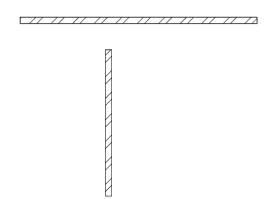
• Click on icon (representing T connection) on Toolbar then select with a single click the wall to be adjusted (1), then the second wall (2).
