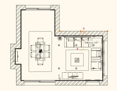
Before creating a wall elevation view it is also possible to select a part of the highlighted wall to be used for the snapshot:
