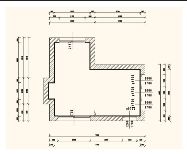
The dimensions will follow the changes of the drawing. You can add new ones to the current or delete existing ones. You can also move dimensions in groups later in case the location is incorrect. This method is as it follows:
