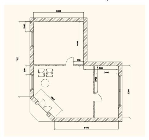
What you can see on your screen now, that is a favoured layout of ARCHLine.XP® so called the Split View. When you create the first element that has an equivalent in 3D, the program automatically displays it in the 3D model window. This split layout helps continuously monitoring how your design appears in 3D view, which is created on the floorplan.
