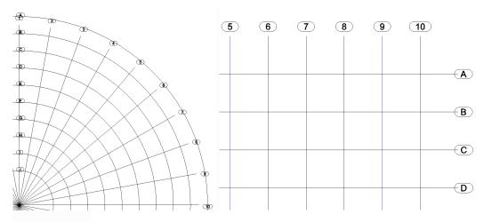
ARCHLine.XP automatically links objects, column, beam, to gridlines or intersection point of two gridlines. It means moving a gridline, ARCHLine.XP also moves the position of the linked elements to keep them at the gridline intersections.
