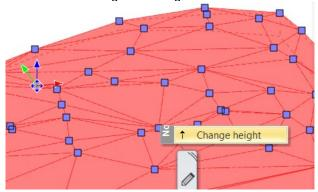
By default, the command changes the elevation of the selected node only. If you wish to add hill or valley you have to switch off the Move terrain points only checkbox. See below.
