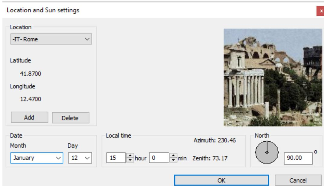
We had defined the location on Earth with orientation as we want to see the sunlight effect on a specific date and time. We can display the sunlight and shadows with proper settings and then we can adjust the sunlight effect periodically by changing the date and time.
