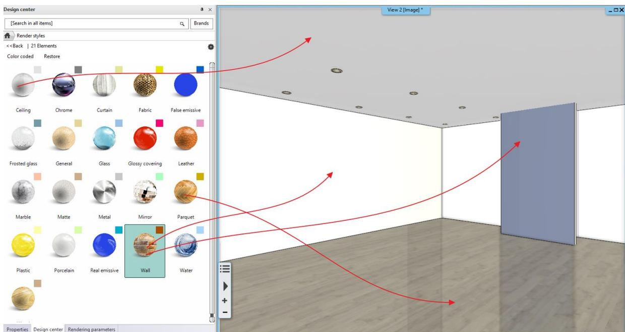
On 3D model using "Colour code" representation mode we can quickly check if we didn't leave any surface out.
