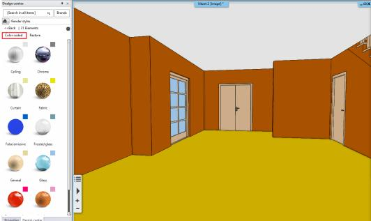
This visualizes the model re-colored by the color-codes of the material render styles applied to their surfaces. You can easily find all glass or metal surfaces for example and if a surface has a different color code than the tiny color swatch at the left top corner of a render style you can click and drag the proper one onto that surface to change it.
